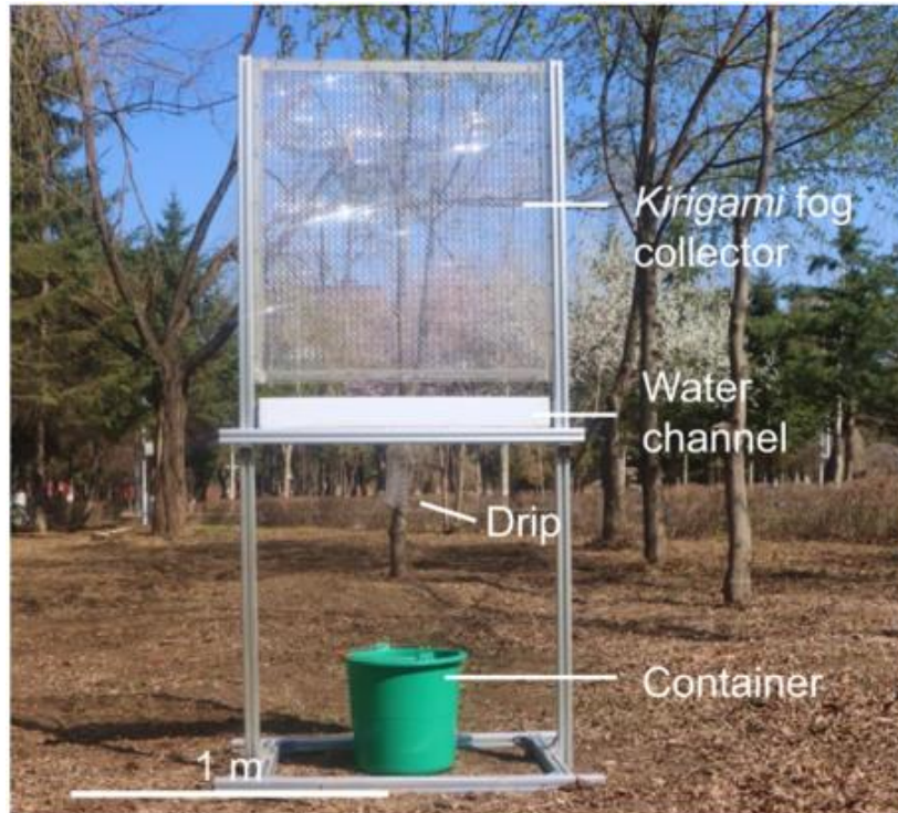
Figure 1. Fog Collection System [6]
